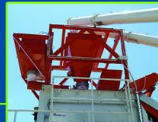
Cement & water scale
